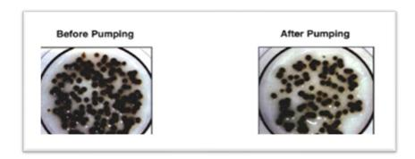
The Nova Rotors pump ensures a high efficiency of the separator, causing almost no damages to the oil droplets and no risk of creating emulsions that are hard to separate.
