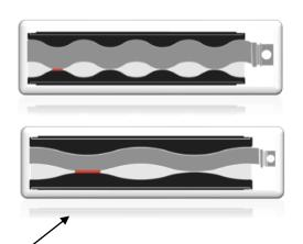
Short-pitch and long-pitch rotors for multi-stage or maximum flow pumps. Available in materials and with surface treatments for wear and corrosion resistance.
