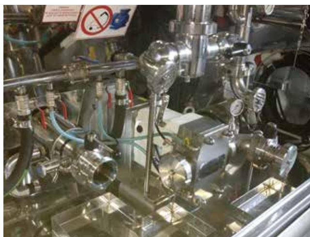
Pumped liquid - transporting syrups, chocolate, etc. Pump - LPX80-1 installed on a truck cistern
